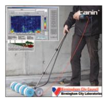
**Birmingham City Laboratories (BCL)** has recently invested in new test equipment to undertake 12,000m<sup>2</sup> of half-cell potential mapping of a large multi-storey car park.
